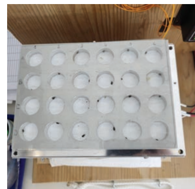
Cold plate arenas where insects are cooled down to reach a specific temperature, prior to thermophysiology tests.
