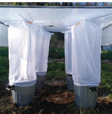
Setup for one replicate of the combined impact experiment with the weevil Bagous nodulosus and the fly Phytoliriomyza ornata .
