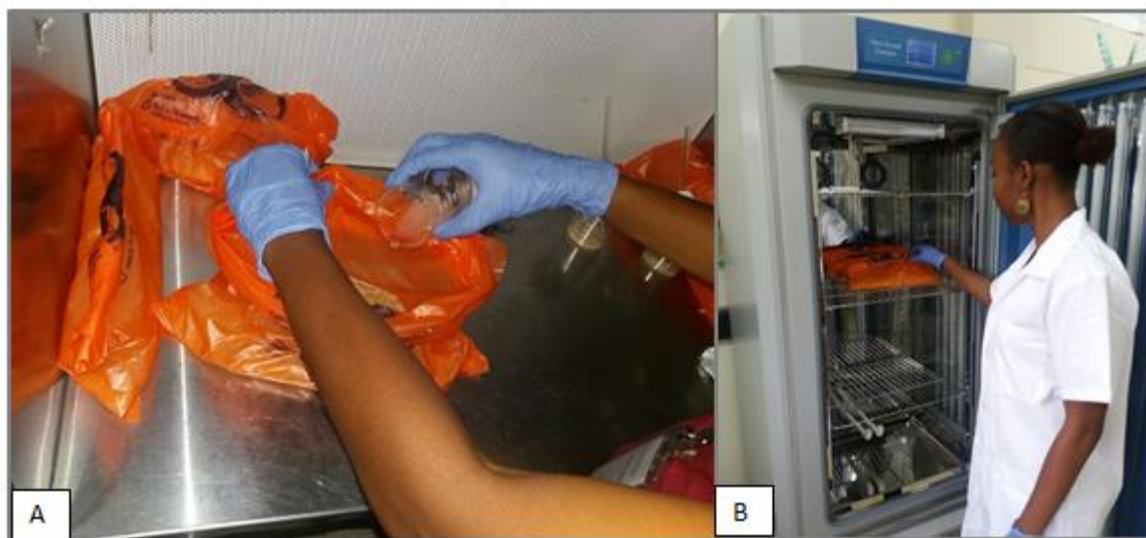
Figure 1A; Inoculating parboiled rice with Beauveria bassiana suspension in autoclavable bags under the laminar flow. 1B; Placement of the inoculated media in sealed autoclavable plastic bags for incubation at 24°C and 85% Relative Humidity in the Plant Growth Chamber at Bodles Research Station.
