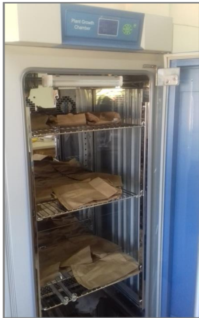
Figure 2; Inoculated rice transferred from autoclavable plastic bags to brown paper bags for drying at 24°C and 85% RH in the Plant Growth Chamber.
