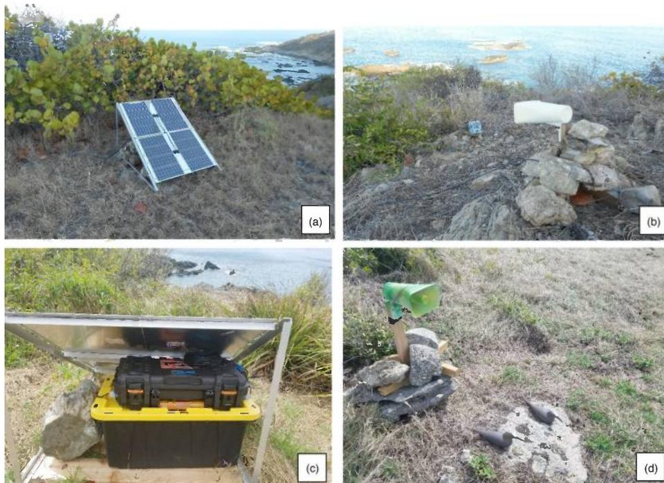
**FIGURE 3** The seabird sound systems on Desecheo Island: (a) solar-powered system; (b) sound system; (c) outdoor speaker with motion-sensing camera pointing towards it; (d) Brown noddy decoy and speaker arrangement
