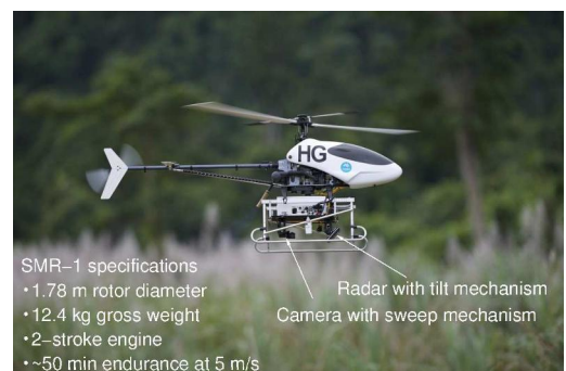
Figure 1. CSIRO SMR-1 helicopter configured for weed survey flights over mountainous rainforest.
