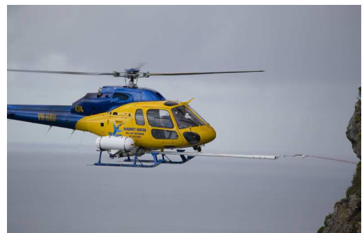
Figure 7. The helicopter mounted – forward lance spray apparatus provides simultaneous detection and treatment of outlier weeds (ground asparagus and bitou bush) on sheer cliffs. The spray pods have a 200 litre capacity. With the lance extending beyond the rotor blades, downwash is limited and foliar spray treatment is targeted.
