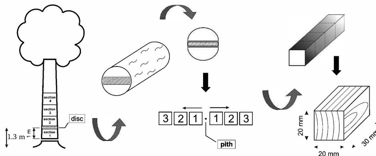
Fig. 1. Tree sampling and position of testing samples in the tree
