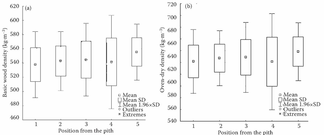
Fig. 3. Variation in the basic density and oven-dry density in the radial direction from the pith to the bark in the stem of Turkish hazel
