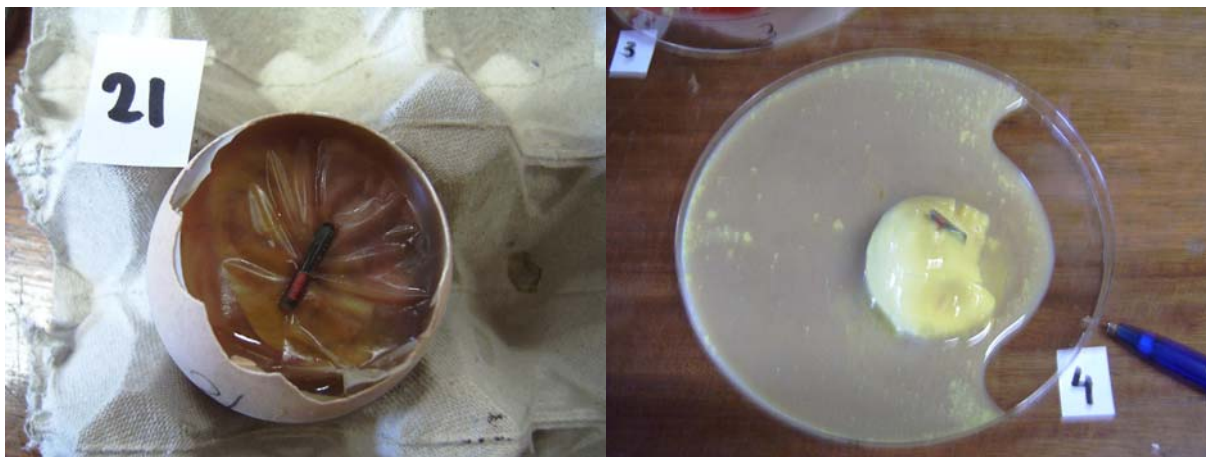
Figure 1 Temperature transponder in the air cell of an egg (left) and temperature transponder on a firm and smelly yolk (right)
