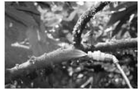
Figure 1. CFValve™ (GATE LLC, USA) spray management valve in use with a directional cone spray (D2-45 nozzle combination). Results indicate that such combinations could improve frosty pod control by maximising dose transfer (R.P. Bateman)
