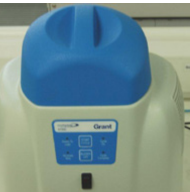
The Stirling cycle controlled-rate cooler allows for optimal cryopreservation of important cultures (photo A. Kermode)
