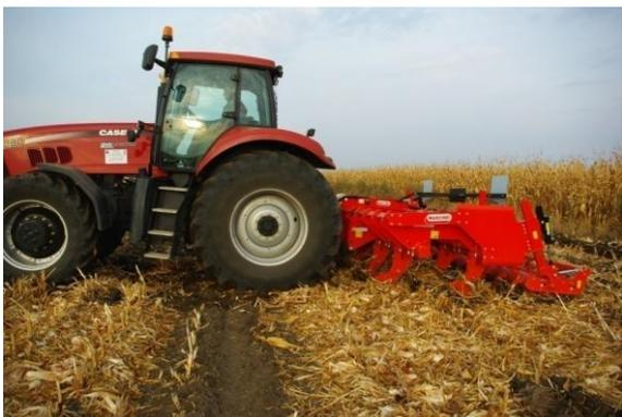
Fig. 8: Grubber, working depth 0.25 m
