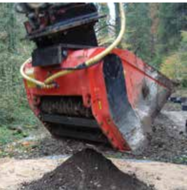
Rhizome crushing treatment (photo: E. Gerber)
