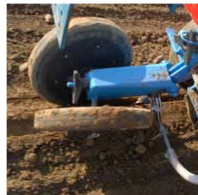
Nematode application equipment on a maize sowing machine developed by cult-tec of Freiburg in Germany, www.culttec.de/nematec-projekt.html (photo: M. Lichtenberg, e-nema, Schwentinental)
